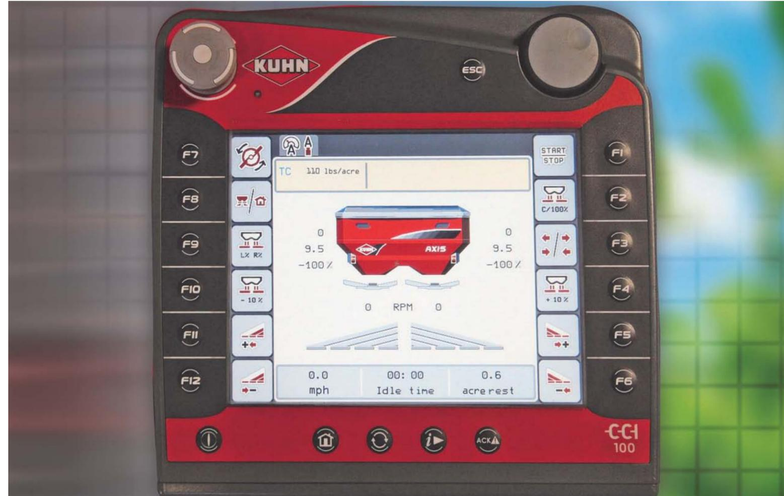
Please note that with the optional Kuhn CCI 100 with activated CCI Command (Section Control) and CCI Control the functions required for all premium H-EMC features are met. The GPS receiver is required to be purchased separately.
