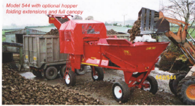
Model 544 with optional 料斗 folding extensions and full canopy | 544 机型，带可选料斗折叠扩展结构域全覆盖式顶盖
