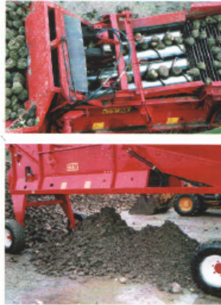
Model 544 with optional 料斗 folding extensions and full canopy | 544 机型，带可选料斗折叠扩展结构域全覆盖式顶盖
